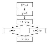
This is an example of a **control-flow graph** (**CFG**). Nodes are instructions, and edges represent the possible flow of control: if there is an edge from  $n_1$  to  $n_2$ , then control can flow directly from  $n_1$  to  $n_2$ .
